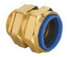
RADI-E1W/E1WF double compression industrial glands are excellent weatherproof glands designed to-be-used in highly robust environment. These glands offer an IP66 rating seal for both inner and outer jackets of the cable. They also provide excellent armor locking and effective earth continuity. RADI E1WF glands are flameproof glands designed for used in flammable environment. Typetested to BS EN 50262:1998+A1:2001+A2: 2004. Marine application approved product by ABS.
