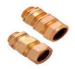
**RADI-PBPG** single compression cable glands are manufactured from high quality yellow brass with nickel plating. The onion-ring seal are made of either neo-print or nitrate rubber providing an IP54 rating seal on the outer cable jacket. This gland is suitable for use with all types of non-armored cables in dry indoor environment.
