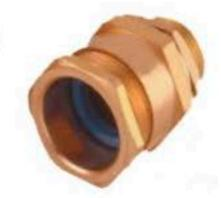
RADI-RXT industrial cable gland provides the same functional properties as the RADI-A2 cable gland except it is specially designed to-be-used with braided armored cables. Clamping the wire braid onto the gland provides excellent electrical continuity. The gland provides good mechanical cable retention with an IP66 environmental sealing. Type-tested to BS EN 50262:1998+A1:2001+A2: 2004. Marine application approved product by ABS.
