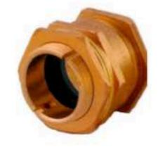
RADI-BWR is a three-part gland developed for securing single wire armored (SWA) cables in indoor and dry environment. The positive armor locking increases the mechanical strength and effective earth continuity. The gland has an IP54 environmental seal rating. Type-tested to BS EN 50262:1998+A1:2001+A2: 2004. Marine application approved product by ABS.
