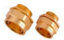
RADI-CWR/(CW) single compression industrial glands provide an IP66 rating environmental sealing on the outer jacket of a single wire armored (SWA) cable, making it suitable for applications in out-door and/or out-door wet environment. This weatherproof gland offers positive armor locking, effective earth continuity and tight liquid and/or moisture sealing. Type-tested to BS EN 50262:1998+A1:2001+A2: 2004. Marine application approved product by ABS.
